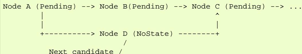
The Taskmaster first evaluates the nodes A, B, and C and starts building some children of node C. Assuming, that the maximum parallel level has not been reached, the Taskmaster will examine Node D. It will find that Node C is a pending child of Node D.
